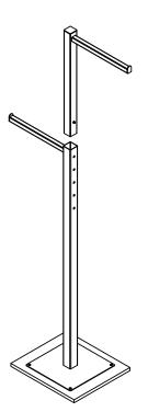
3. Insert top of unit into post, lining up popout button with holes. Adjust height using the holes on the side of the post.
